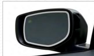
**Auto-Dimming Exterior Mirrors with Approach Light.** When you approach the vehicle or unlock the doors with the keyless entry system, LED lights in each exterior mirror illuminate the ground next to and towards the rear of the vehicle. During nighttime driving, the Auto-Dimming Exterior Mirrors dim in unison with the Auto-Dimming (Interior) Mirror when glare is detected.
