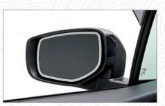
Auto-Dimming Exterior Mirrors with Approach Light. Designed to enhance nighttime driving safety by reducing headlight glare. Upon approaching the vehicle or unlocking your doors with the keyless entry system, LED lights in each exterior mirror illuminate the ground next to the vehicle's doors.
