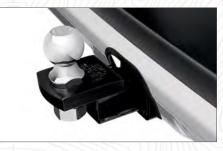
Trailer Hitch. Heavy-duty 2-inch receiver rated at 3,500 lbs. towing capacity, 350 lbs. tongue weight for the 2.4L Turbo XT and Outback Wilderness models, and 2,700 lbs. towing capacity, 270 lbs. tongue weight for the naturally aspirated 2.5L.
