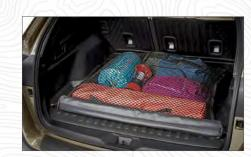
Cargo Net. Neatly holds cargo and prevents it from sliding while the vehicle is in motion. Either anchor it to the sides of the cargo area to help prevent shifting from front to back or lay it across the floor to help keep things from rolling around.
