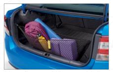
Cargo Net. Neatly holds cargo and prevents it from sliding while the vehicle is in motion.
